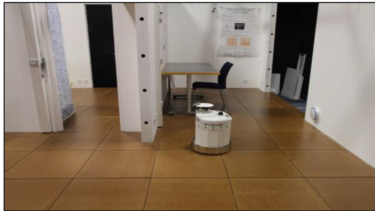
Figure 2.26 – PeKeelII robot communicating with an interactive sensing floor.
