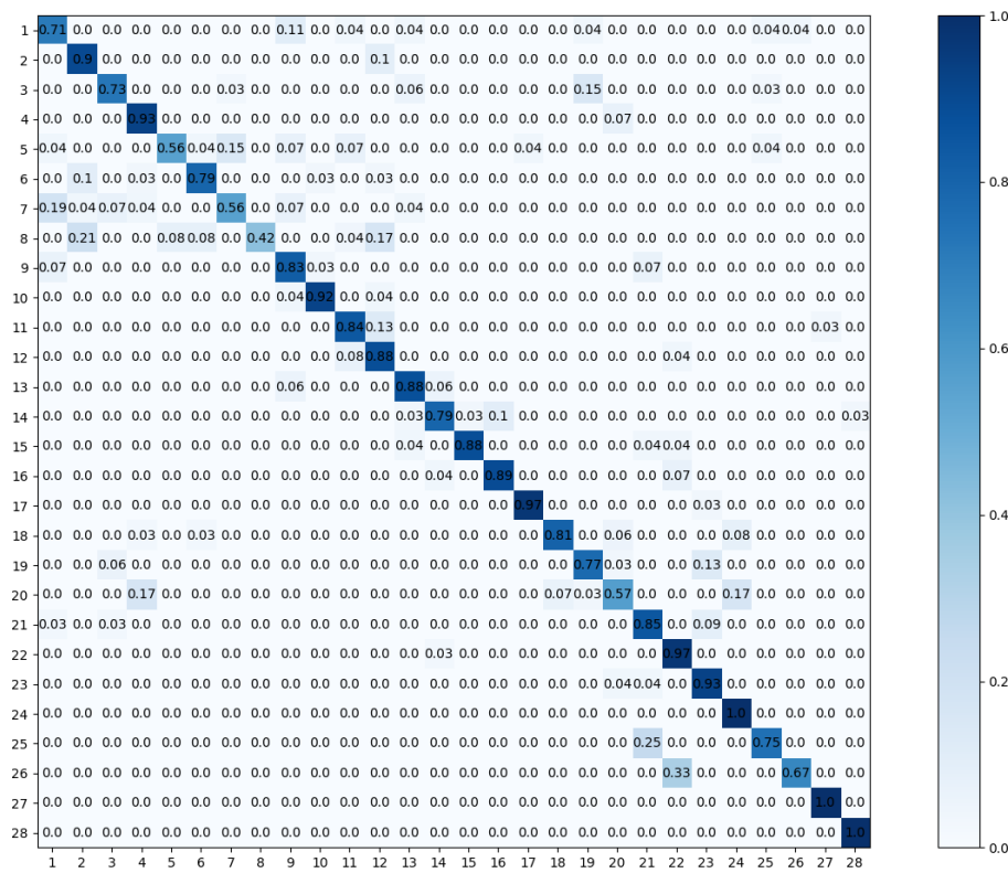
Figure 5.29 – The confusion matrix obtained on the Online DHG dataset for the task of online recognition of 28 gesture types. Labels of gestures can be found in Table 5.3.
