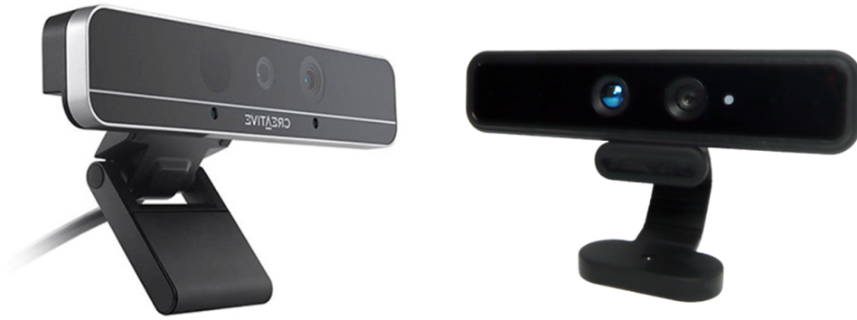
Figure 2.8 – Example of short range RGB-D sensors. Left: Intel RealSense SR300 [117], right: SoftKinetic DS325 [135].
