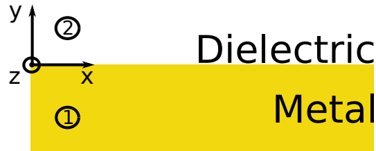
Figure 2.19: Sketch of the geometry for SPPs propagation at a planar interface between a metal and a dielectric medium.
