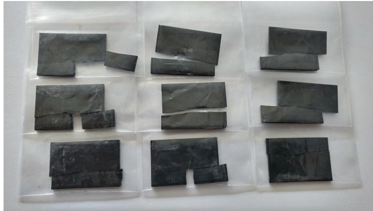
Figure 4.39: Ceramics broken during cutting or polishing procedures
