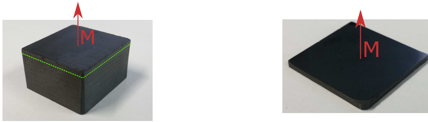
Figure 3.25: Photos of original block of the Fb6N sample with highlighted preferred magnetization and cut direction and a thin sample after the cut.
