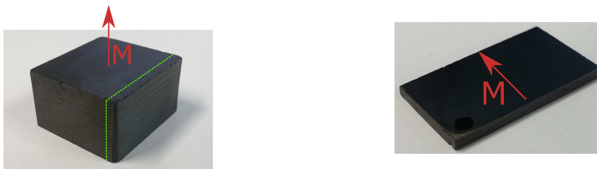
Figure 3.34: Photos of original block of the FB6N sample with highlighted preferred magnetization and cut direction and a thin sample with in-plane \mathbf{M} after the cut.
