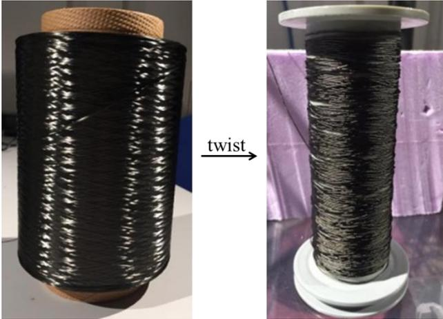
Figure 2-28 TORAYCA® FT300 carbon fibre and twisted thread.
