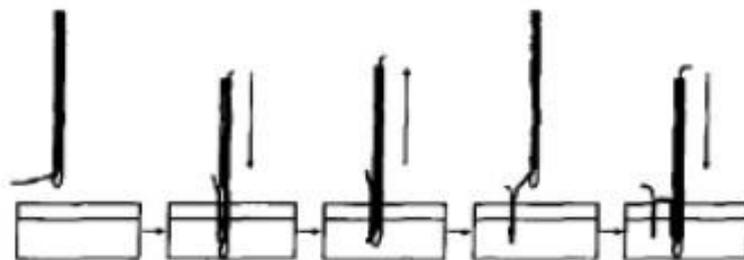
Figure 2-4 Tufting technology: Aerotiss<sup>®</sup> 03S. [7]
