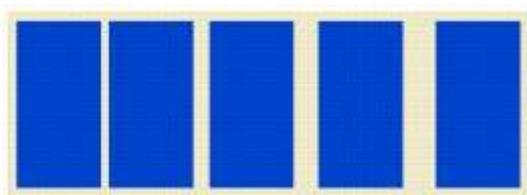
**Figure 48:** Transmission line measurement structure
