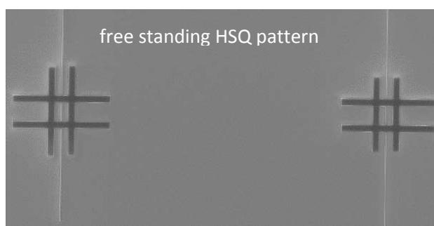
**Figure 56:** Example of a free-standing HSQ structure after Ammonium hydroxide based solution and supercritical drying.
