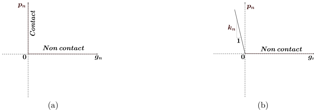
Figure 1.10: Graphical representation of contact laws: Penetration is not allowed in Kuhn tucker condition (a) while in the penalty method (b) contact constraints are violated and penetration depends on contact pressure
