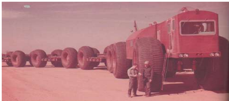
Figure 1.5: Application of articulated wheeled vehicle (one of the R. G. LeTourneau trackless trains LCC-1) [17].
