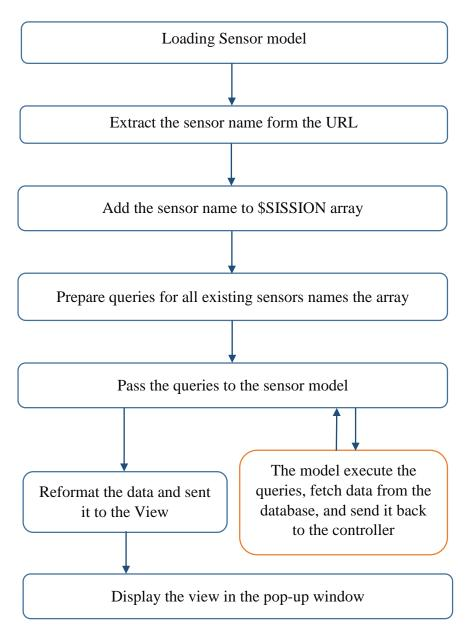
Figure 5.8: A flow chart for multi\_statistics function
