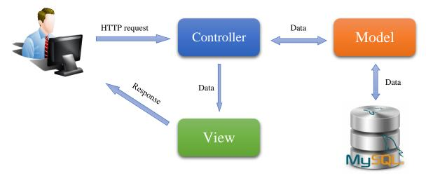
Figure 5.3 : Model-View-Controller pattern
