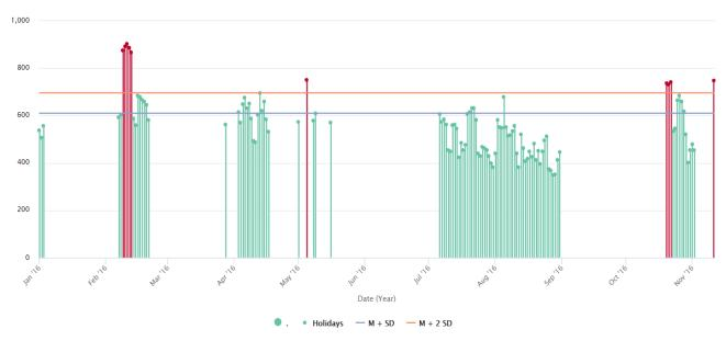
Figure 4.49: High probability of leakage detection during the holidays
