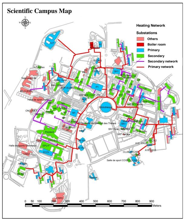
Figure 3.6: The heating network in the campus
