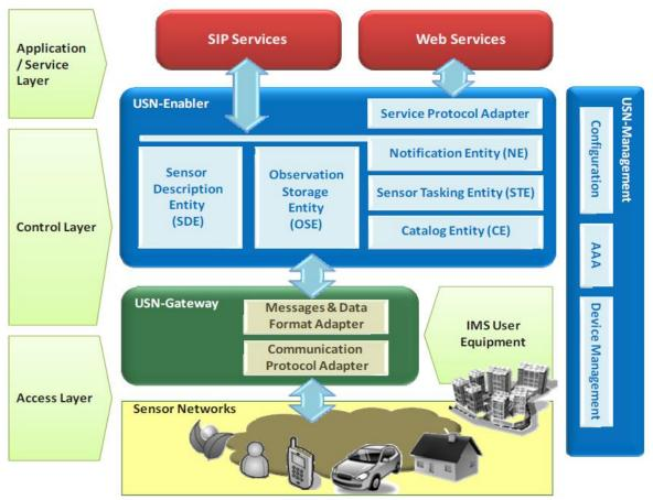
Figure 2.7: The architecture of USN platform
