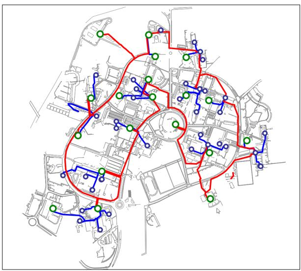
Figure 3.7: The electrical grid in the scientific campus
