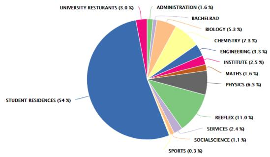
Figure 4.41: The distribution of the water consumption for the sub-meters in 2016
