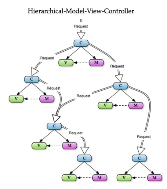
Figure 5.4: Hierarchical-Model-View-Controller pattern (Source: inviqa.com)
