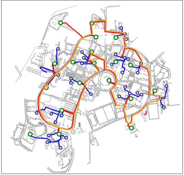
Figure 3.8: Fiber optic communication network (in yellow)
