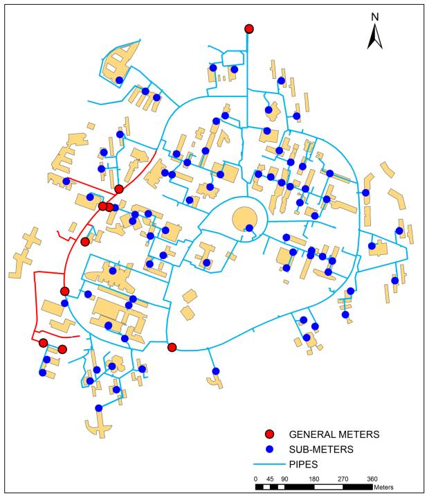
Figure 3.5: Distribution of the general and sub-meters in the campus
