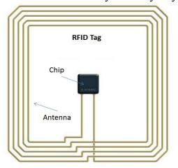
Figure 2.2 : Radio Frequency Identification
