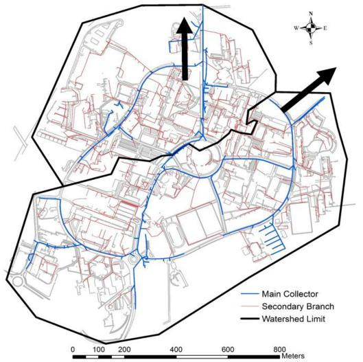
Figure 3.11: The stormwater system with watersheds limit
