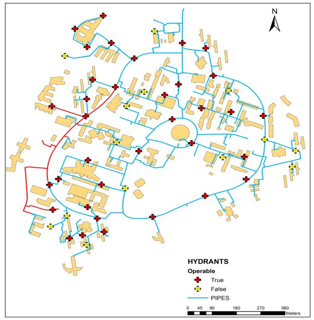
Figure 3.3: Pipes and hydrants distribution in the campus
