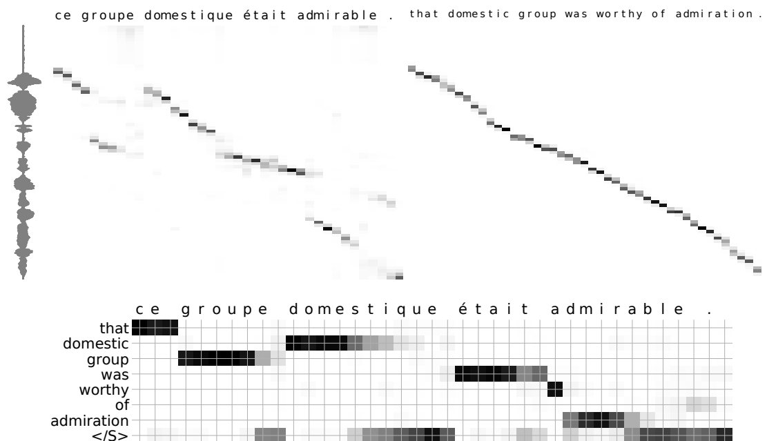
FIGURE 5.5: Examples of forced alignments performed by the pre-trained AST model (top left), the ASR model (top right), and MT model (bottom). To better visualize the character-level outputs, the alignments are reversed: the x-axis corresponds to the target sequence and the y-axis to the source sequence.
