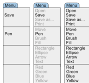
Figure 2.14: Illustration of Role 14: Ephemeral adaptation progressively reveals content in menus based on history—adapted from [Fin+09].
