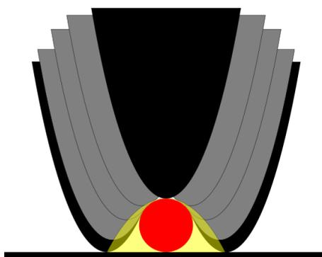
Figure 2.12.: Illustration of the convolution artifact. A parabolic tip is represented (black and gray) as it is scanned over a sample (red). Assuming a constant deflection, the recorded height corresponds to the height of the end of the tip, which might (black) or might not (gray) be the actual point of contact between the tip and the sample. The resulting image, the path of the end of the tip, draws the yellow shape, the convolution of the tip and sample shape.
