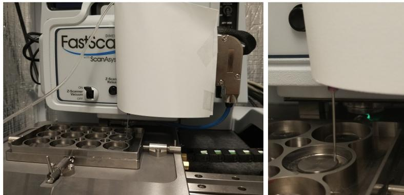
Figure 9.4.: Pictures of the fluid exchange needle, held at a fixed position from the head allowing it to be lowered in the different wells while keeping the probe holder in a safe area and vice-versa.
