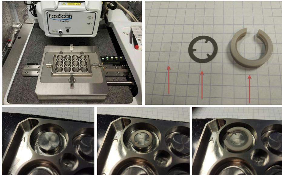
Figure 6.1.: Multi-Well Plate Setup. Top left: empty Multi-Well plate on the FastScan. Top right: coverslip (left), spring (middle), and spring clamp (right). Bottom: zooms on well A1 with the successive placement of the coverslip (left), spring (middle) and spring clamp (right).
