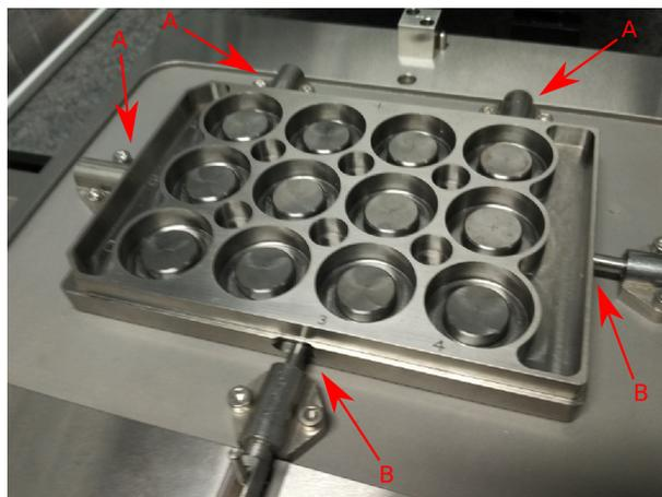
Figure 6.2.: Multi-Well positioning. The lateral placement of the Multi-Well is controlled by 3 adjustable ball-headed screws (A) and two retractable springs (B).
