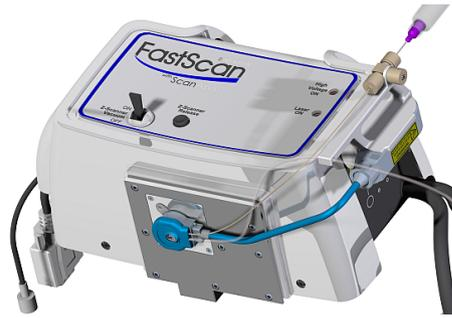
Figure 9.3.: Fluid apparatus on dimension FastScan head. Fluid intake from the top right through the thin flesh-colored tube, blue fluid chamber to host the cantilever in fluid, larger transparent fluid outtake leaving on the right. © Bruker
