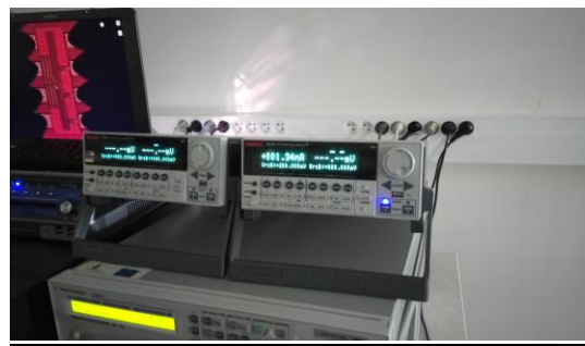
One Keithley 2636A connected to VSS.
