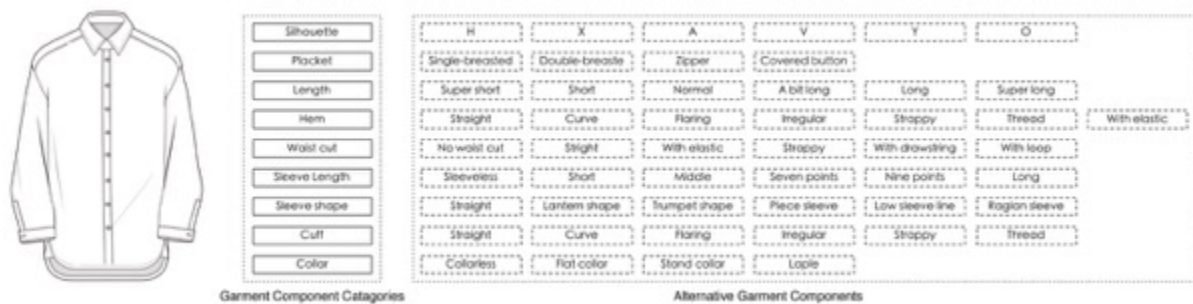
Figure 2-14: Garment Components Module (GCM) of a shirt: Garment component Categories and their alternative garment components.
