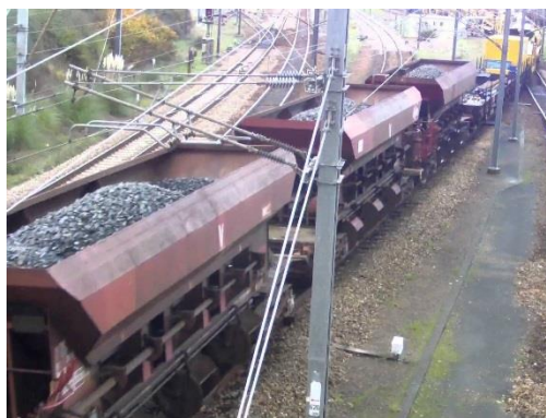
Figure II. 22: Wagons trémies [refw5].
