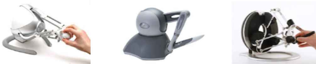
FIGURE 2.2: Examples of haptic kinesthetic devices (From left to right: Novint Falcon® [4], Phantom Omni [5] and Omega® [6])
