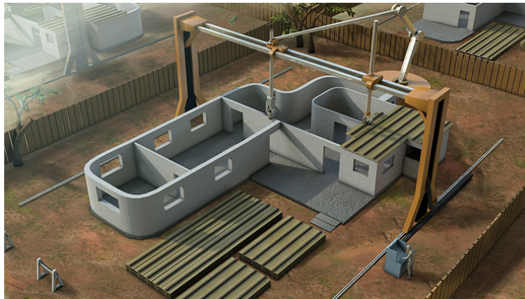
Figure 2.9 – Southern California University 3D printing machine
