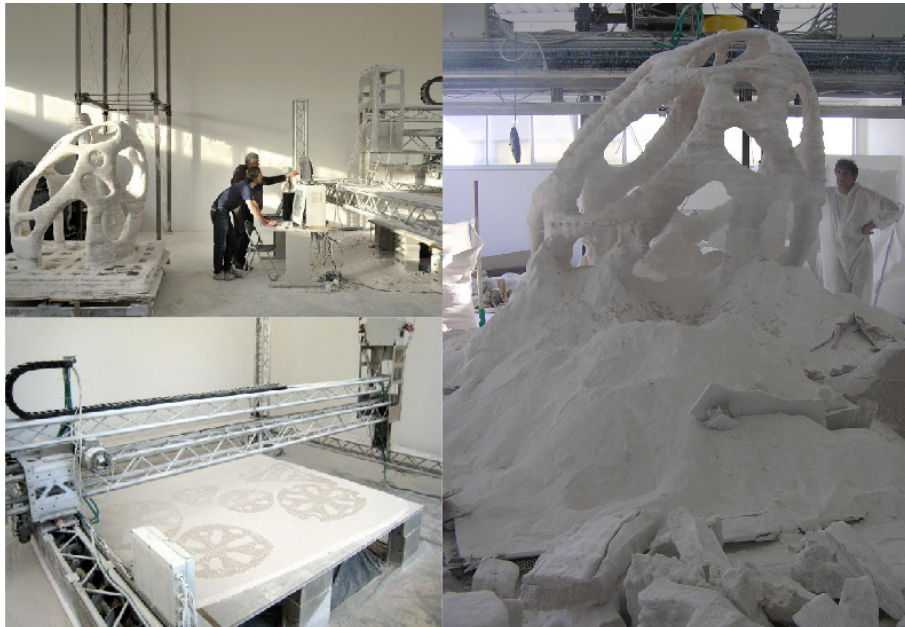
Figure 2.2 – D-Shape : Solidification from sand
