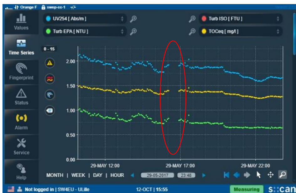
Figure 3.3. Loss of S::CAN data at Polytech'Lille on May 29, 2017.
