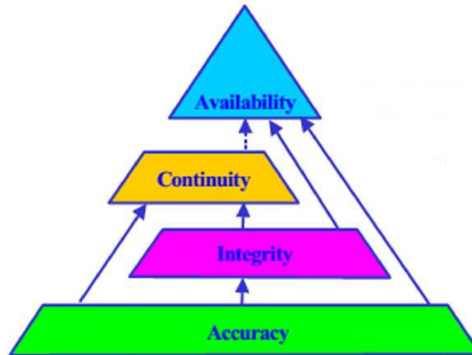
Figure 1.1 – GNSS Required Navigation Performance (RNP) Parameters for Aviation Navigation
