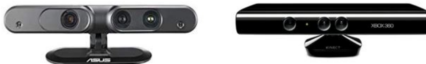
FIGURE 1.4 – Depth cameras: ASUS Xtion PRO LIVE (left) and the Microsoft Kinect (right).
