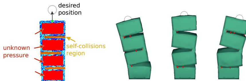
Figure 4.12: Soft tower with four cavities actuated with pressure. The algorithm determines how to inflate each cavity to get the end-effector reach the desired position (white sphere). Self-collision points are represented by red lines.
