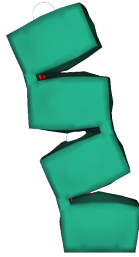
Figure 4.13: Pressure estimation. Two positions on the soft object are controlled, the tip and the middle.
