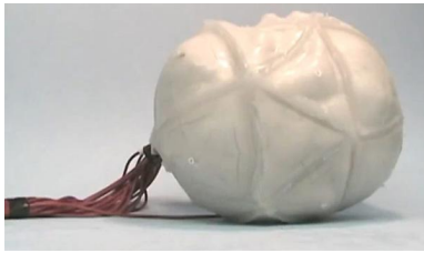
Figure 5.7: Spherical soft robot proposed by Steltz et al. (2009, 2010) (image from their paper). The robot is composed of 20 cells around its outer perimeter (each cell being filled with jamming material), and a central actuated cavity.
