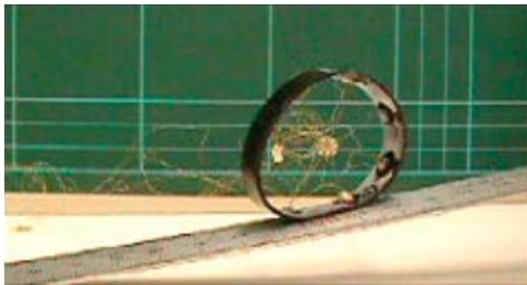
Figure 5.3: Soft robot proposed by Sugiyama & Hirai (2006) (image from their paper). The robot is actuated with eight SMA coils.
