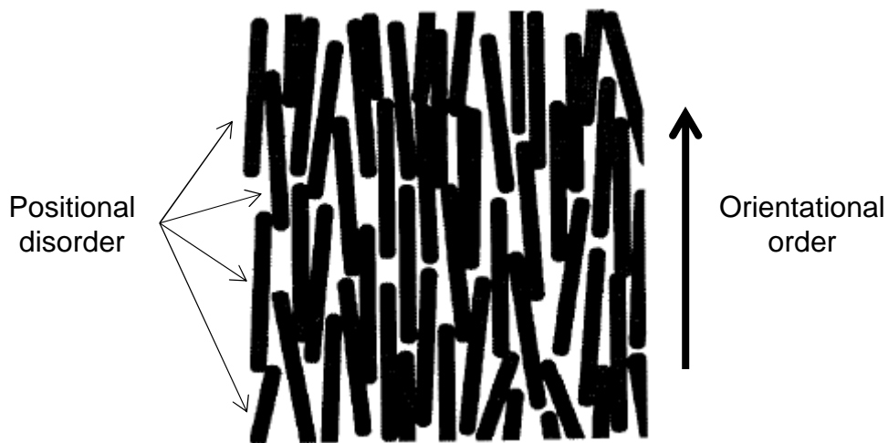
Figure 1.5. Structural representation of a liquid-crystalline polymer.
