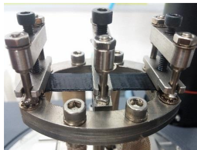
Figure 9 Dual cantilever test for nanocomposite 3D printed layers
