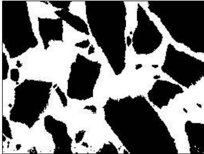
Figure I-2. The characteristic function I(\mathbf{x}) of a cross-section of the cemented granular media in figure I-1
