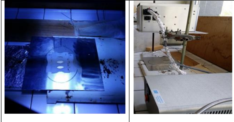
Figure II.2-3: expérimental set up for UV irradiation (Dymax flood 2000)
