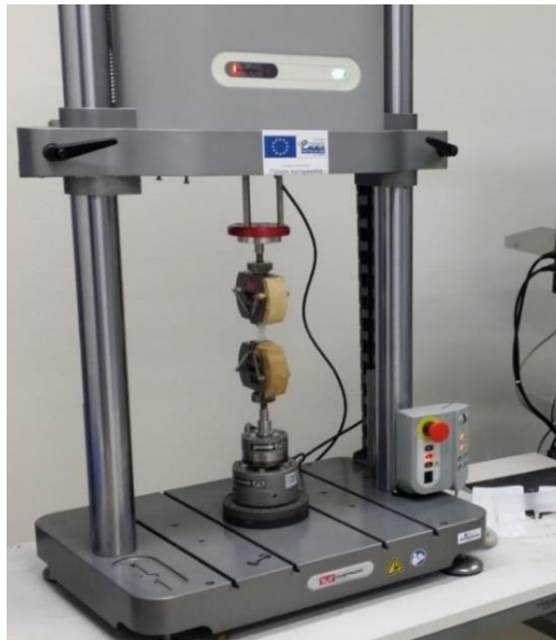
Figure II.1-3: Machine de traction ElectroPuls E3000
