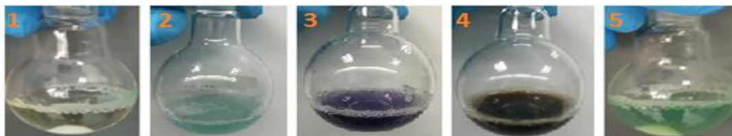
Figure 1: Colour changes at different stages during the synthesis of CuS-BSA nanocomposite. 1: BSA aqueous solution, 2: BSA- Cu^{2+} metal ion complex formation, 3: growth of BSA- Cu^{2+} at pH 12, 4: Nucleation of Cu^{2+} - S^{2-} on BSA, 5: Growth of CuS-BSA.
