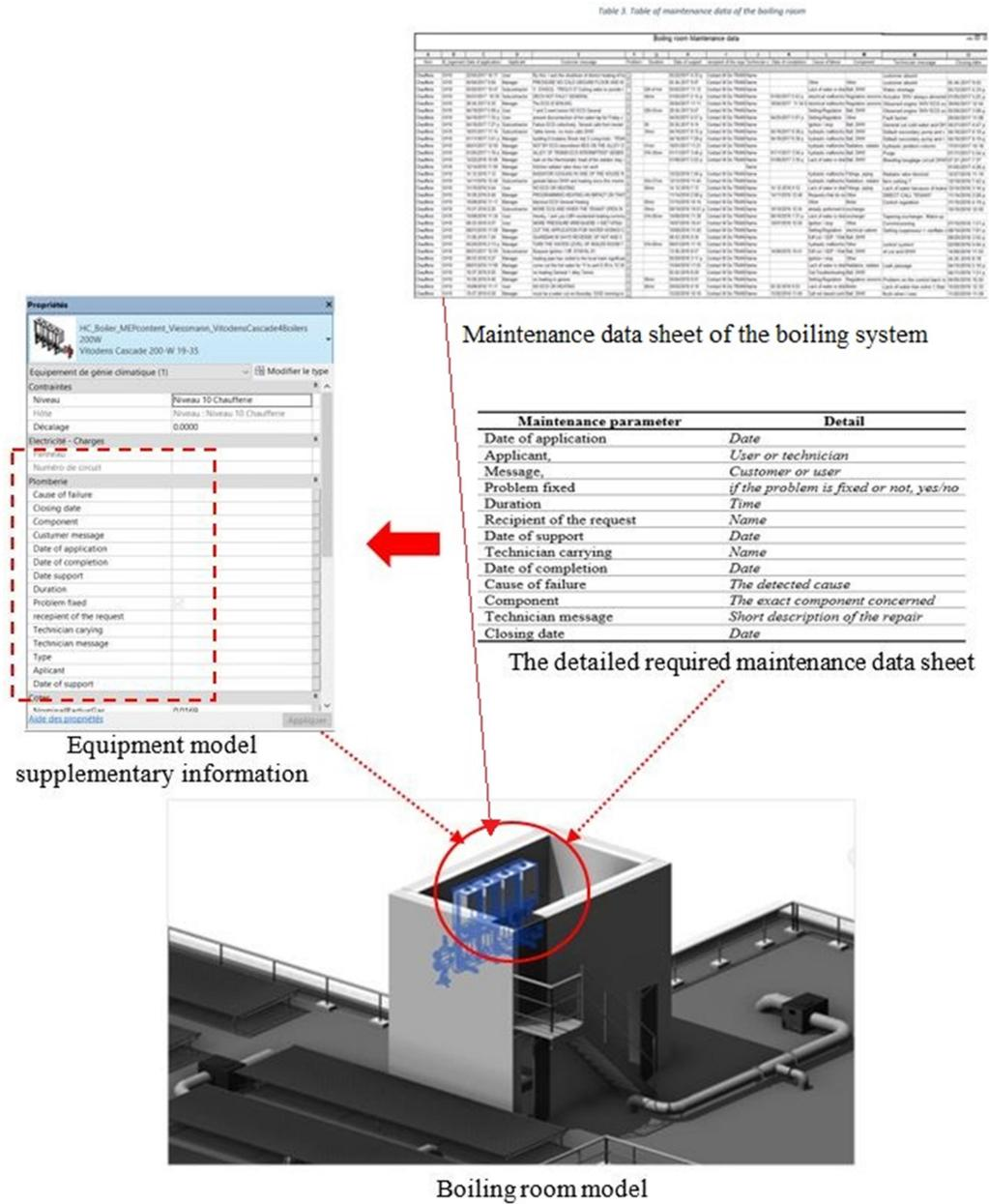
Figure 3.23. Building asset maintenance with BIM model (Alileche and Shahrour, 2018)
