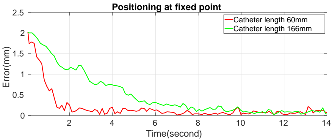
Figure 5.7: Convergence of positioning errors with different catheter length (60mm and 166mm).
