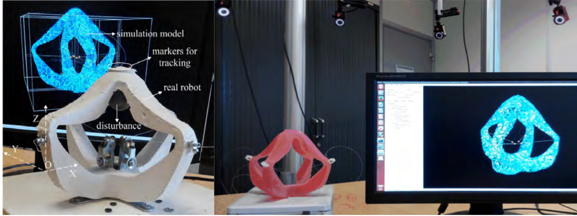
Figure 3.6: Experimental setup for the position control of soft robots. Two soft parallel robots with different Young modulus ( 150kPa for the white robot in the left figure and 240kPa for the pink robot in the right figure) are tested. The left robot is used for the experiment of the first closed-loop control and the right one for the second implementation. Both robots have four soft legs and are actuated by cables. The simulation model serves as a simulation-based predictor. The 3D position of the end effector can be obtained by the position perception system.
