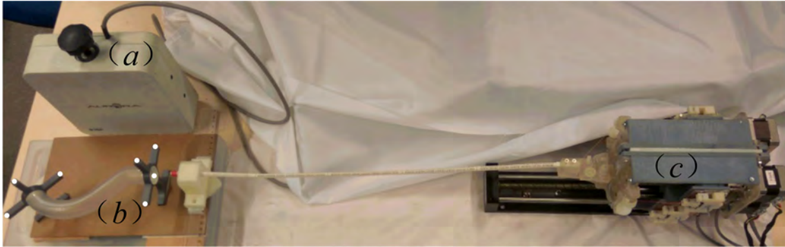
Figure 5.4: Experimental setup for the motion control of a catheter robot through contacts. (a) NDI electromagnetic tracking system: Aurora; (b) a rigid tube for the experiment. The white points are the feature points which are used for the calibration; (c) the cable-driven continuum catheter robot which has four step motors to actuate the bending and one step motor to control the insertion.
