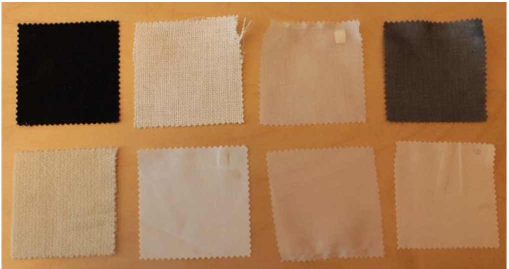
Figure 4. Fabric swatches (Top, left to right: Wool Barathea, Cotton Mousseline, Linen Heavy, Polyester Chiffon. Bottom left to right Wool Basket weave, Silk with elastane, Linen Holland, and Polyester Sateen)
