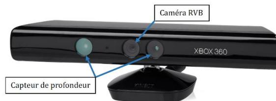
**Figure 4. 8 :** Caméra Kinect.
