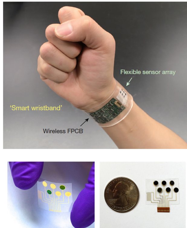
Figure 1.8 – A smart wristband integrating flexible sensors presented in [Gao et al. (2016)].
