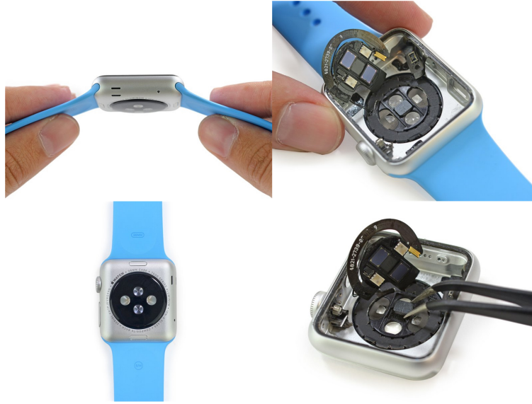
Figure 1.7 – Illustration of the Apple Watch with sensors perfectly integrated inside the back of the watch structure [iFixit].
