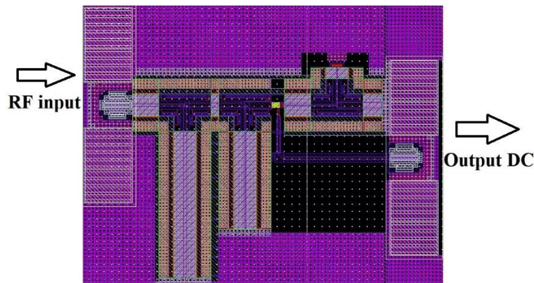
Figure 4.31 The layout of the frequency compensated detector in the G-band.
