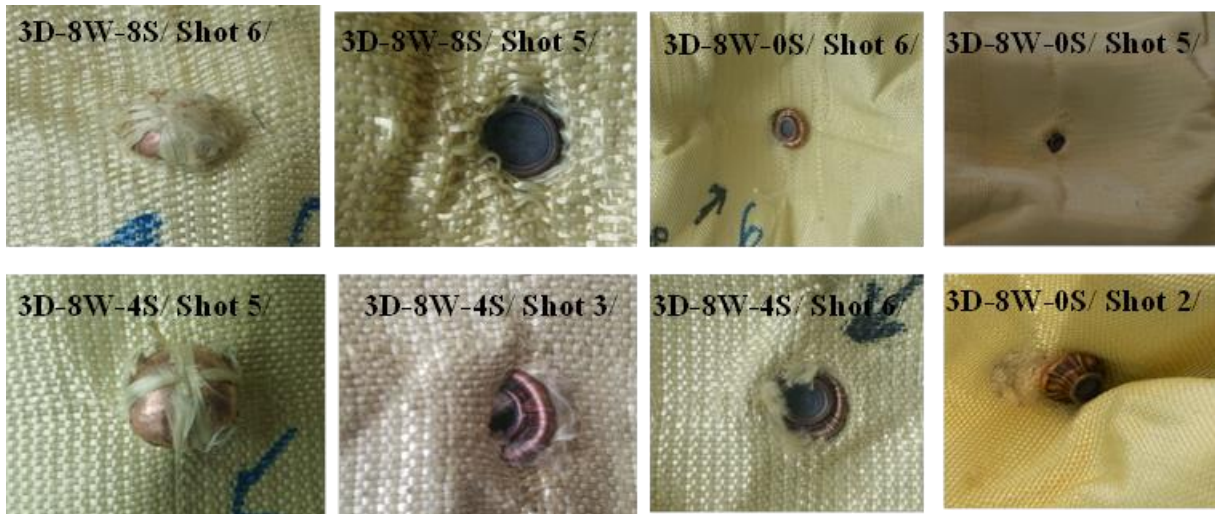
Figure 7.9 Examples of the trapped projectiles in some sample panel
