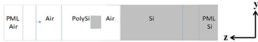
Figure 2.3: (a) 3D schematic representation of the PC films (Si/Air/Si structure) made of ridges of width L and height h . (b) Projection of the unit cell used for the FEM calculation.
