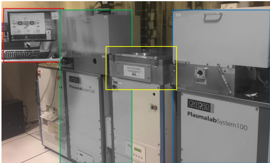
Figure 2.13 – Oxford Instruments Plasmalab 100 Plus ICP-RIE. Chamber one (blue box), chamber two (green box), load lock (yellow box) and controller (red box).
