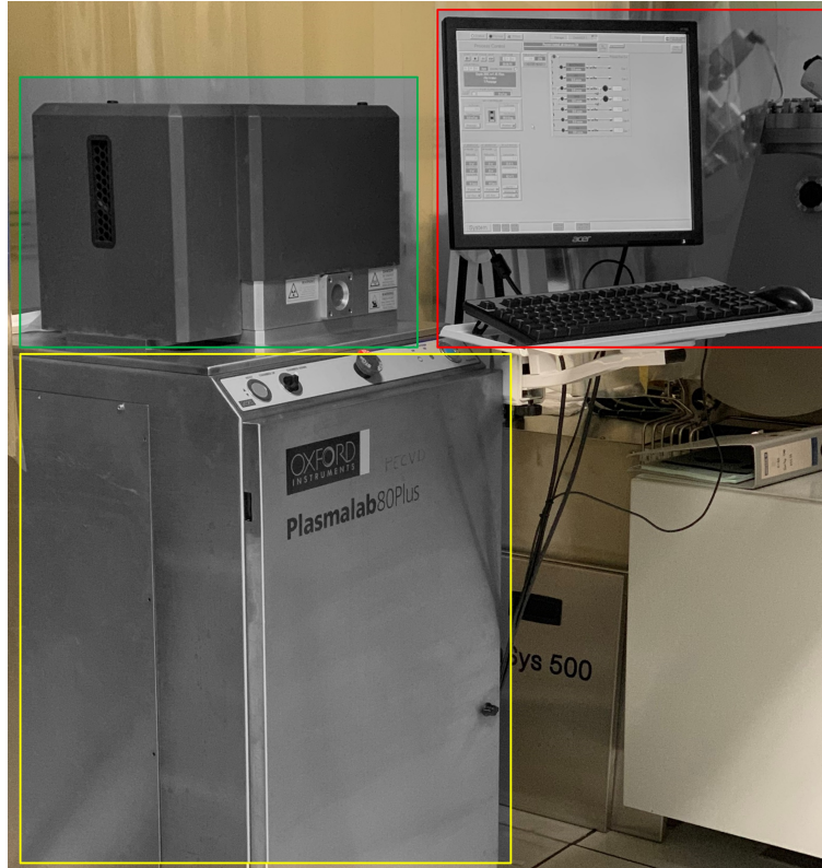
Figure 2.4 – Oxford Instruments Plasmalab 80 Plus PECVD. Main chamber (green box), pumps and electronics (yellow box) and controller (red box).
