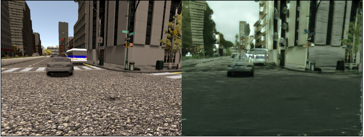
Figure 2.9 – Sim-to-real unsupervised transfer (M.-Y. Liu, Breuel, and Kautz, 2017) from synthetic images of the CYNTHIA dataset (Ros et al., 2016) to realistic images of the CITYSCAPES dataset (Cordts et al., 2016).
