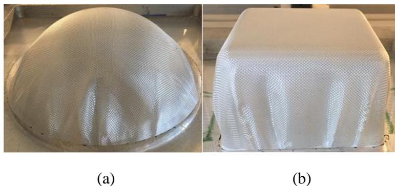
Figure 3.10 Wrinkling phenomenon in (a) hemispherical and (b) square-box forming
