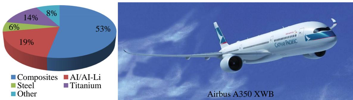
Figure 1.1 Weight fractions of materials processed in the Airbus A350 XWB[5]
