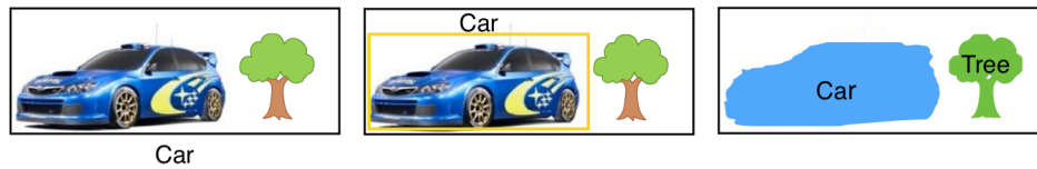
Figure 2.1: From left to right: image classification, detection, and segmentation tasks. The image classification is about assigning a category to an image, detection classifies and localizes an object, while segmentation asks for a more detailed scene representation. The figure is imported from (Malinowski, 2017)
