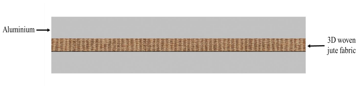
Figure 2.10. 2/1 lay-up configuration used for FMLs fabrication
