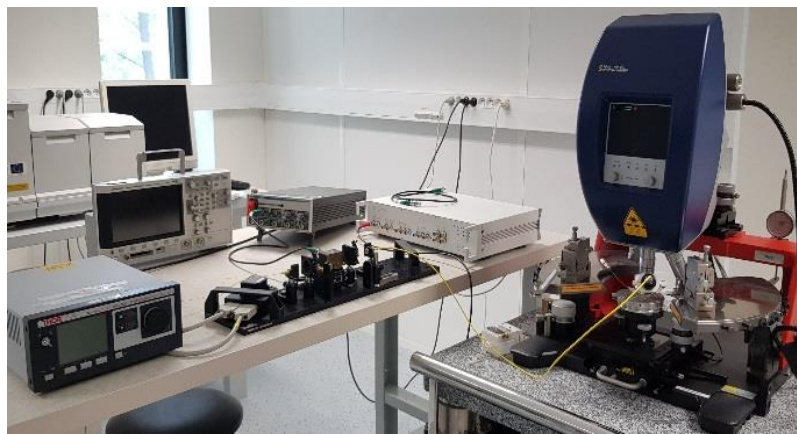
Figure III.3.3 Photograph of the PT excitation and LDV detection setup
