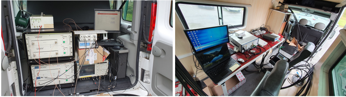
Figure 5.33: Base station in one laboratory truck and mobile station in the second laboratory truck
