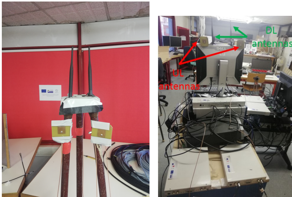
Figure 5.5: Base station and mobile station setup from left to right respectively
