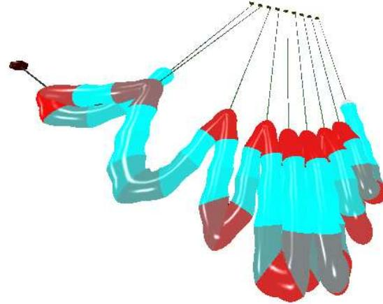
**Figure 3. An example of spline segment coloration using our curvature isolation process, during interactive sweep deformation. Darker segments correspond to those that the algorithm selects as high curvature ones.**
