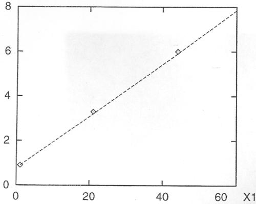
Figure 4: Maximal values for  $\log(u'_{\max})$  on axis  $x_2 = 0$ . Numerical values obtained with linearized Euler equations (points). Theoretical exponential growth rate  $-k_i$  (line).
