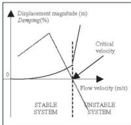
Fig. 2. Critical flow velocity generating structure instability development.
