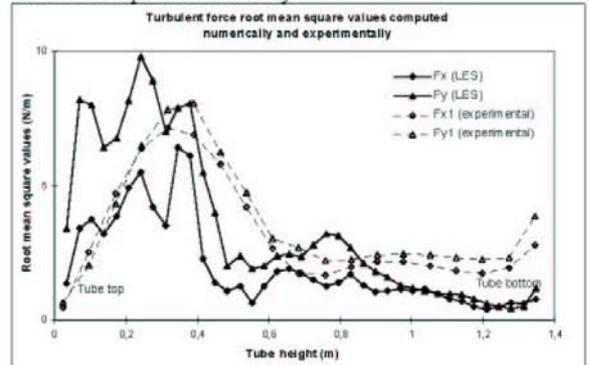
Figure 6 : Turbulent force root mean square values along the tube (N/m) :  $F_x$  and  $F_y$  components computed numerically (lines) and experimentally by Granger and Perotin (points).
