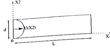
Fig. 1 Mean flow profile  $U(y)$ . Inlet disturbances are imposed in section  $x = 0$ , and nonreflecting conditions in section  $x = L$ .
