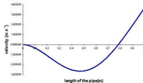
Fig. 6 - Shape of the second fundamental mode of the structure
