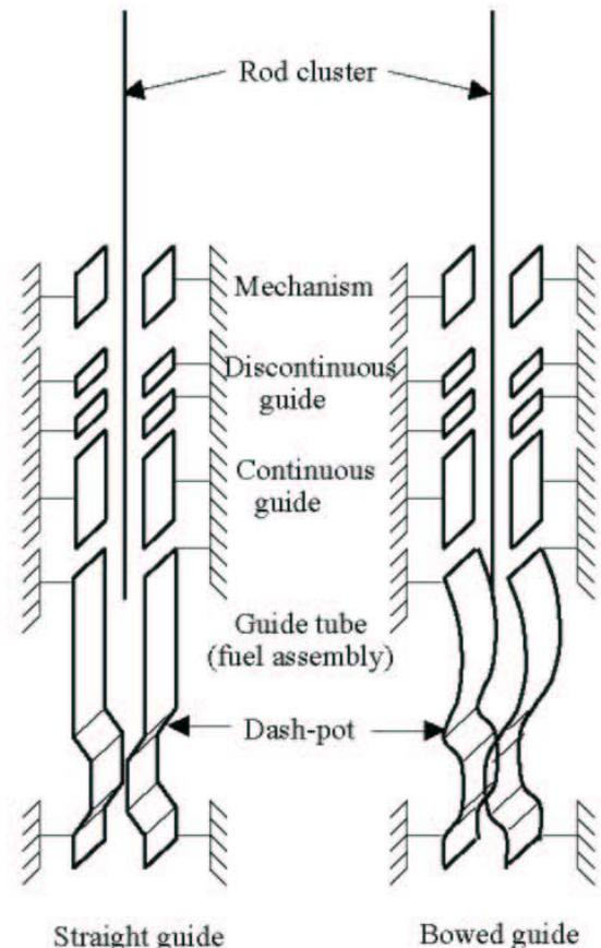
Figure 1 : schematic view of the numerical model.
