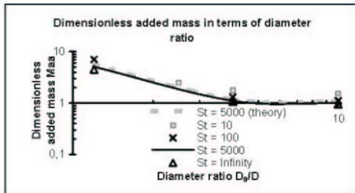
Fig. 14: Dimensionless added mass in terms of diameter ratio for concentric tubes for different Stokes numbers for viscous fluid ( $St = 10, 100, 5,000$ ) and nonviscous fluid ( $St = \infty$ ). Comparison of numerical and available analytical solutions for  $St = 5,000$  [25].
