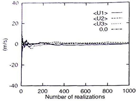
Figure 3: Statistical mean of velocity  $\overline{u_{ti}}$  over 1000 realizations.
