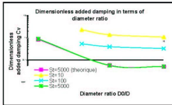
FIG. 7 – Dimensionless added damping depending on internal and external tube diameter ratio for concentric tubes for several Stokes numbers for viscous fluid ( $St = 10, 100, 5000$ ). Good agreement between numerical (Longatte et al. [7]) and analytical solutions of Chen [2]
