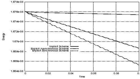
Figure 8. Comparison of fluid structure mechanical energy for three code coupling schemes explicit synchronous, explicit asynchronous and implicit
