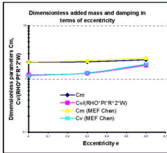
FIG. 9 – Dimensionless added mass and damping depending on the eccentricity for eccentric tubes. Good agreement between numerical solution obtained with a numerical partitioned procedure (Longatte et al. [7]) and numerical monolithic solution obtained with strong coupling (Chen [2])
