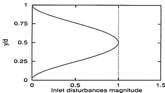
Fig. 2 Nature of inlet disturbances: —, two first modes, and ----, plane mode.
