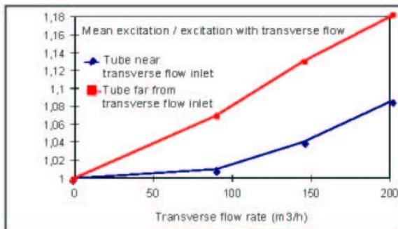
Figure 14 : Comparison of excitation RMS magnitudes with and without transverse flow, for tubes located near and far from the transverse flow inlet 1300 Mwe.
