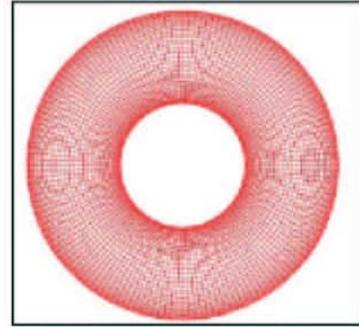
Figure 1 : Fluid mesh for a concentric moving tube.
