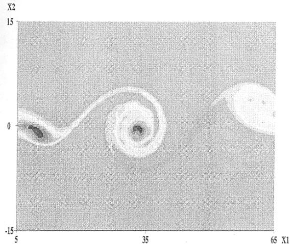
Figure 11: Shear layer non linear development. Vorticity computed with semi-linearized Euler equations.
