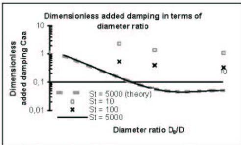
Fig. 15: Dimensionless added damping in terms of diameter ratio for concentric tubes for different Stokes numbers for viscous fluid ( $St = 10, 100, 5,000$ ). Comparison of numerical and available analytical solutions for  $St = 5,000$  [25].
