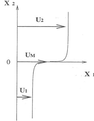
Figure 1: Shear layer mean flow velocity profile :  $U_o(x_2) = U_M \left[ 1 + R_u \tanh\left(\frac{x_2}{2\delta_\theta}\right) \right]$ .
