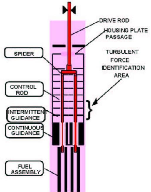
Figure 2: Identification of turbulent forces acting on PWR RCCA near the intermittent guidance bottom.
