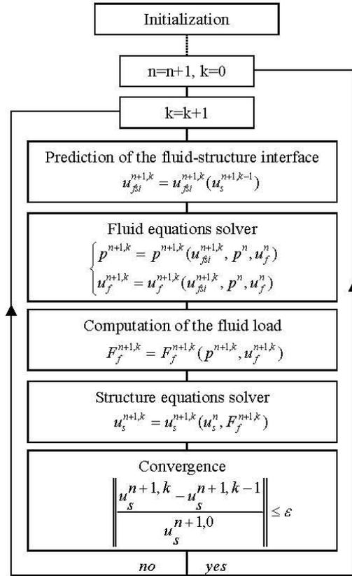
Fig. 2 - Sub-cycling coupling scheme
