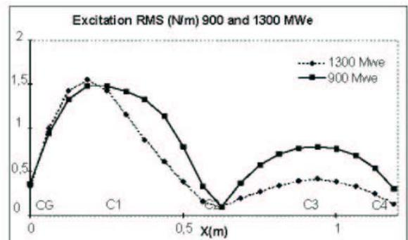
Figure 12: Excitation RMS values for a tube in position E in 900 and 1300 Mwe configurations.
