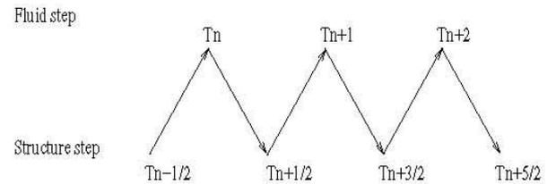
Figure 2. Time progression for an asynchronous code coupling scheme
