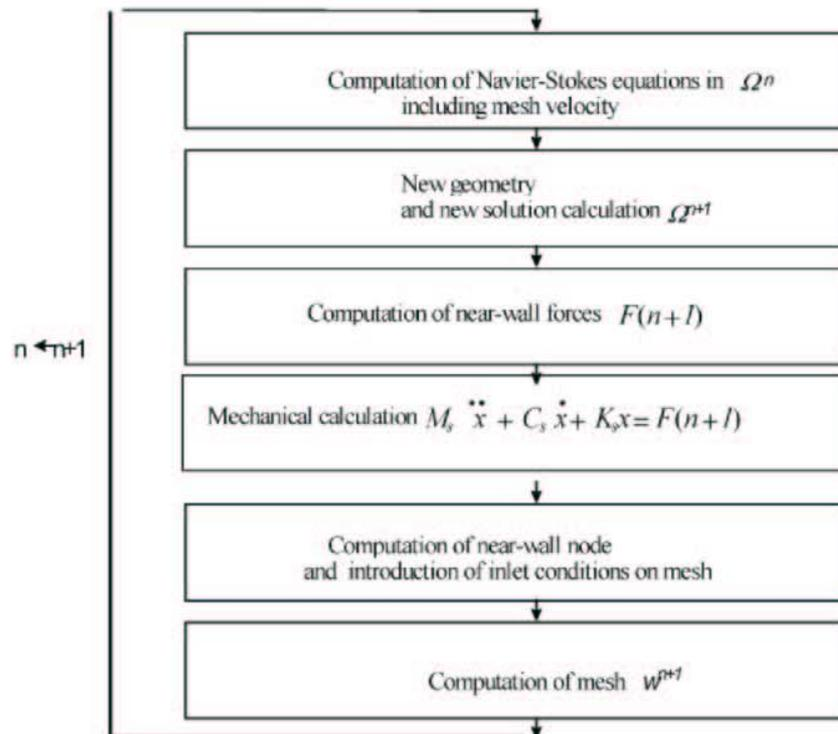
Fig. 4. Computational process for flow and structure motion coupling.
