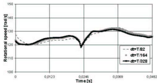
Fig. 10: Comparison of predicted rotating piston velocity versus time using the coarse grid ( $13 \times 90 \times 8$  CV) and various time steps.
