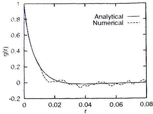
Figure 7: Lateral correlation function  $g(r)$  evaluated numerically and analytically.
