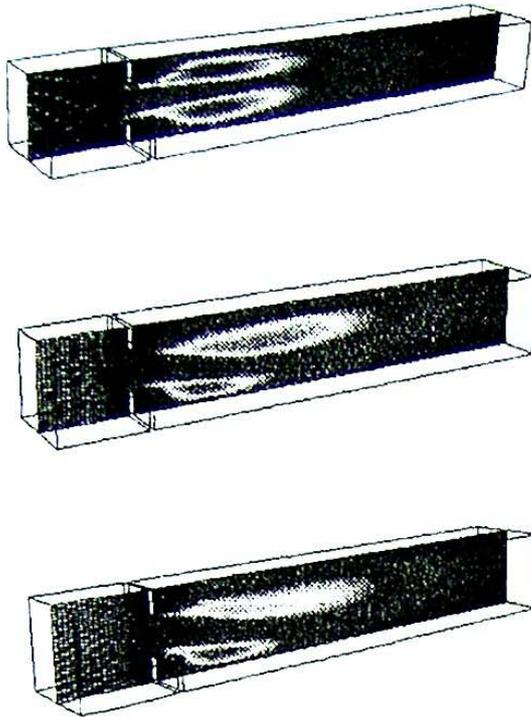
Figure 13: Mean turbulent energy for  $\epsilon = 35\text{mm}$  with  $U_0 = 14\text{m/s}$  (top),  $U_0 = 32\text{m/s}$  (middle) and  $U_0 = 75\text{m/s}$  (bottom).
