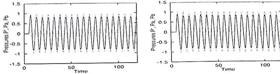
Fig. 8 Time history of pressures  $p'$  (—),  $p_a$  (· · ·), and  $p_b$  (- - -) evaluated numerically (left) and analytically (right) for  $\Omega = 8$  at  $x = \lambda$  with plane mode at the inlet.
