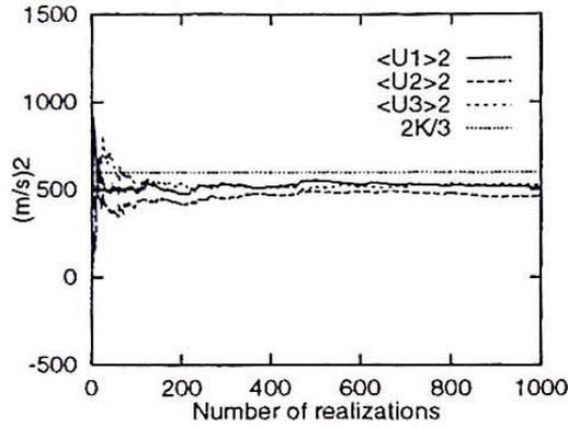
Figure 4: Statistical mean of velocity square  $\overline{u_{ti}^2}$  over 1000 realizations.
