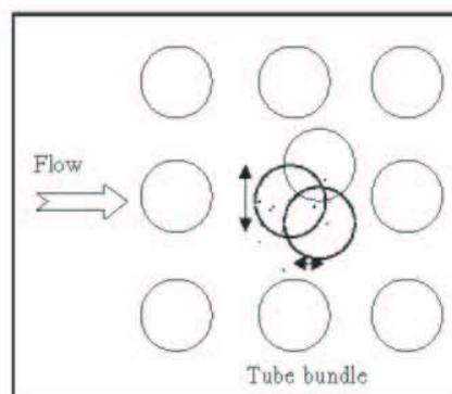
Fig. 1. Lift and drag force effects on a flexible tube belonging to a fixed tube bundle in cross-flow.
