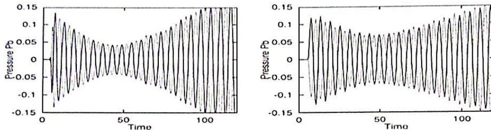
Fig. 12 Time history of pressure  $p_b$  evaluated numerically (left) and analytically (right) with  $M = 0.12$  for  $\Omega = 2\pi$  at  $x = \lambda$  at centerline (---) and at wall (—) with the plane mode at the inlet.
