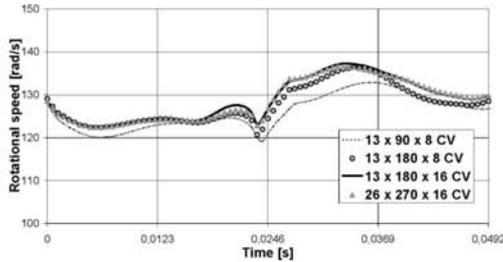
Fig. 11: Comparison of predicted rotating piston velocity versus time using time step  $\Delta t = T/82$  and various grids.
