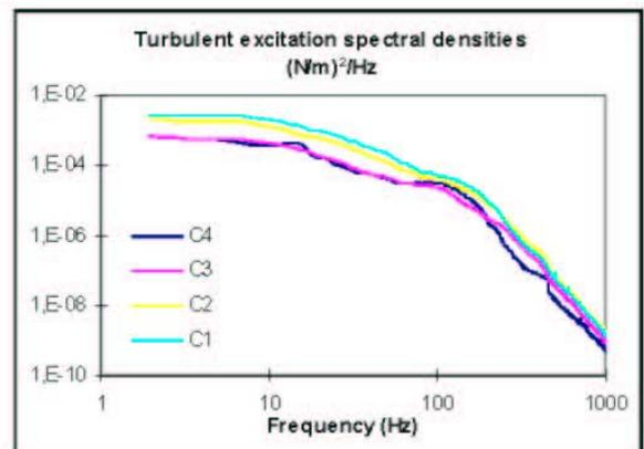
Figure 8: Turbulent excitation spectral densities  $S_{ff}$  of the rod in position E near the first four bottom guide plates (C1 to C4). (900 Mwe)
