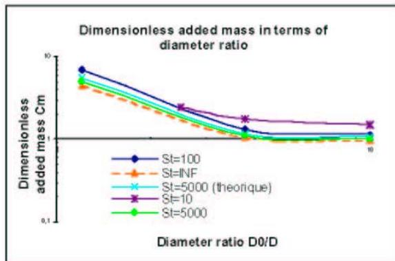
Figure 5 : Dimensionless added mass in terms of diameter ratio for concentric tubes for different Stokes numbers for viscous fluid ( $St = 10, 100, 5000$ ) and non viscous fluid ( $St = \infty$ ). Comparison of numerical and analytical available solutions.
