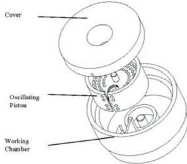
Fig. 4: Three-dimensional view of working chamber and oscillating piston.
