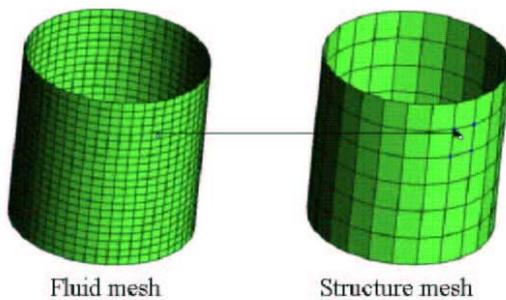
Fig. 4 - Example of non matching fluid and structure meshes
