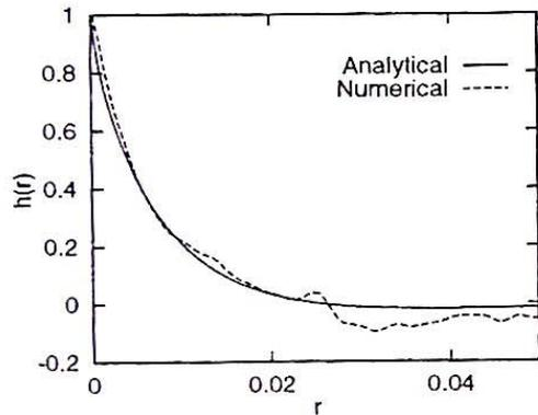
Figure 8: Transversal correlation function  $h(r)$  evaluated numerically and analytically.
