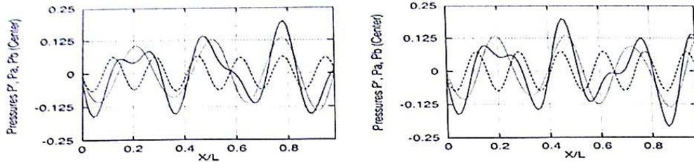
Fig. 7 Spatial propagation of pressures  $p'$  (—),  $p_a$  (· · ·), and  $p_b$  (- - -) evaluated numerically (left) and analytically (right) for  $\Omega = 8$  at centerline with two modes at the inlet.
