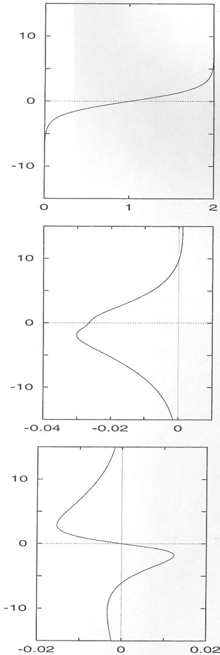
Figure 2: Top : mean flow velocity profile  $U_o(x_2) = U_M[1 + R_u \tanh(\frac{x_2}{2\delta_0})]$ . Middle :  $\Psi$  real part for the unstable mode. Bottom :  $\Psi$  imaginary part.
