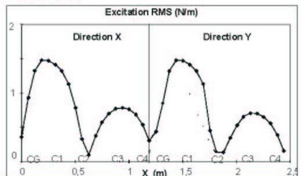
Figure 9: Turbulent excitation RMS (900 Mwe, tube E).
