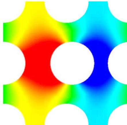
FIG. 10 – Configuration involving a rigid tube moving in a fixed tube bundle represented by a periodic cell including 4 plain tubes
