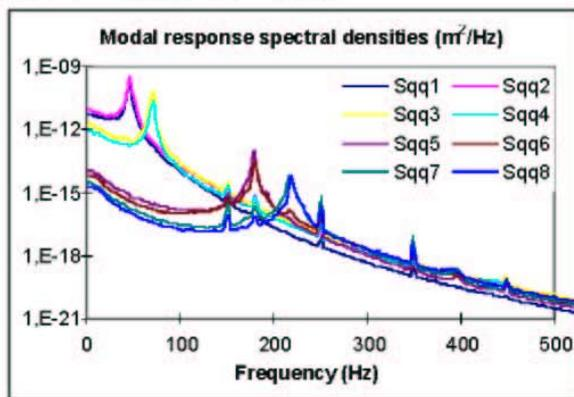
Figure 6: Typical modal response spectral densities  $S_{qq}$  for the rod in position E (900 Mwe).
