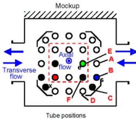
Figure 4: Control rod positions in the intermittent guidance.
