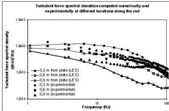
**Figure 8 : Turbulent force spectra  $((N/m)^2/Hz)$  computed numerically (lines) and experimentally (points) at three different locations along the tube at 0.3m, 0.6m and 0.9m from the plate.**
