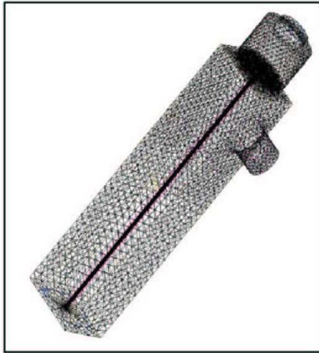
Figure 3 : Wall mesh extracted from the full mesh used for LES: ~45000 P1 nodes, ~200000 elements, near-wall refinement near the tube with 40 wall elements per tube section.
