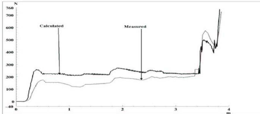
Figure 2 : Comparison of calculated and measured friction forces according to the vertical displacement of the rod.
