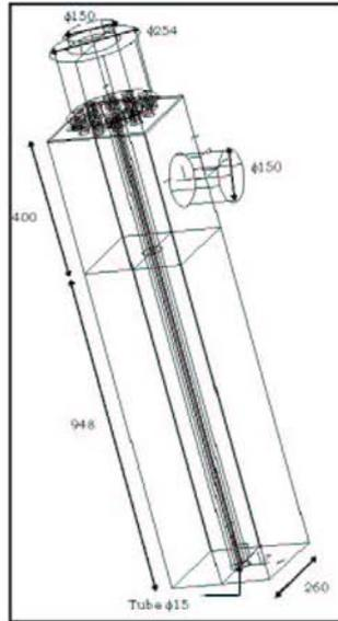
Figure 2 : Test case geometry : a flexible tube ( $\phi$  15 mm) submitted to a complex three-dimensional turbulent axial flow. The test section (260 mm  $\times$  260 mm) is fitted with water inlet at the top ( $\phi$  150 mm), the flow is crossing through a perforated plate and evacuated by a lateral outlet ( $\phi$  150 mm).
