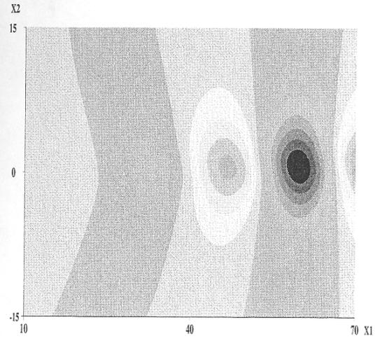
Figure 7: Linear development of unstable mode. Pressure field estimated numerically.
