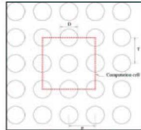
Fig. 16: Computational domain for identification of fluid-structure parameters in a square tube bundle.
