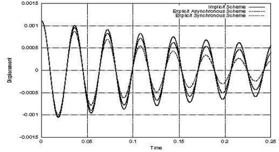
Figure 10. Comparison of structure displacement for different code coupling explicit synchronous, explicit asynchronous and implicit schemes with 896 cells mesh and  $5 \cdot 10^{-4}$  s time step.
