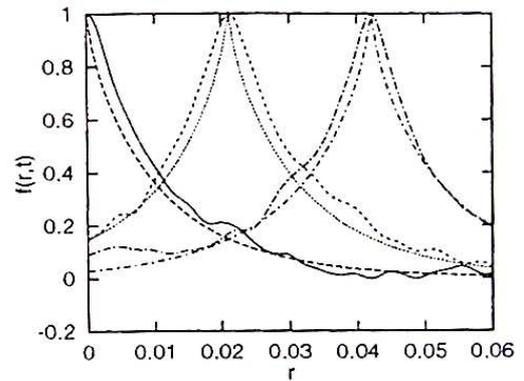
Figure 10: Convection of longitudinal correlation function  $f(r)$  evaluated numerically and analytically.
