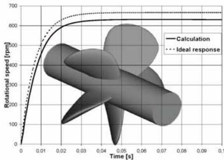
Fig. 12: Dynamic response of the spinner (fluid is water, flow velocity = 1 m/s, initial spinner velocity = 0 rpm,  $\beta = 60$  degrees,  $r = 8$  mm).
