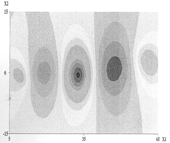
Figure 10: Shear layer non linear development. Pressure field computed with semi-linearized Euler equations.
