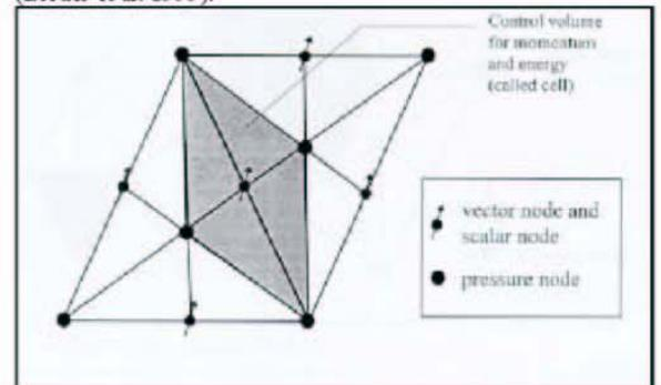
**Figure 1 : P1-non-conforming/P1-iso-P1-bubble element in 2D : pressure nodes in element corners and in the middle of element faces ; velocity nodes in the middle of element faces.**
