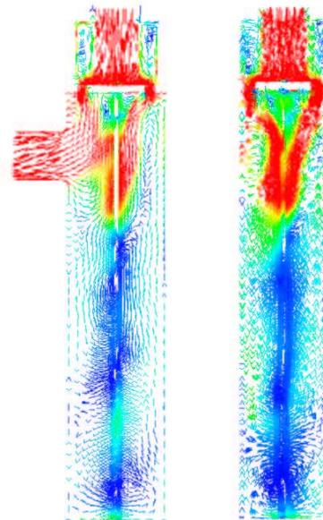
Figure 4 : Velocity mean fields deduced from a time-averaged LES for  $t = 15$  s in the outlet symmetry plane  $x=0$  (left) and in the orthogonal plane  $y=0$  (right). Minimal value : 0 m/s (blue colour), artificial maximal value represented on the graphic: 3,3 m/s (red colour).
