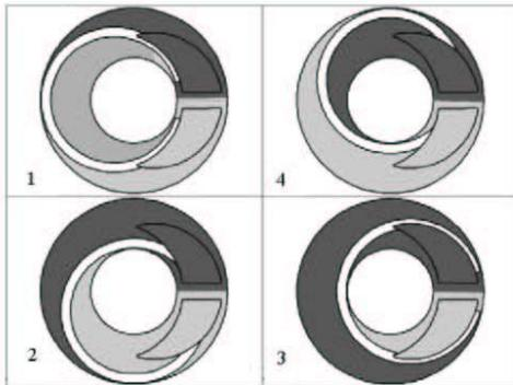
Fig. 8: Piston movement cycle 1-2-3-4. Dark regions represent high-pressure inflow.
