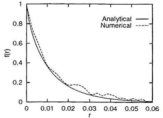
Figure 6: Longitudinal correlation function  $f(r)$  evaluated numerically and analytically.
