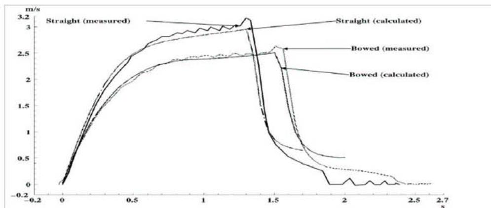
Figure 3 : Comparison of calculated and measured cinematic of the rod drop for a straight and a bowed guide.
