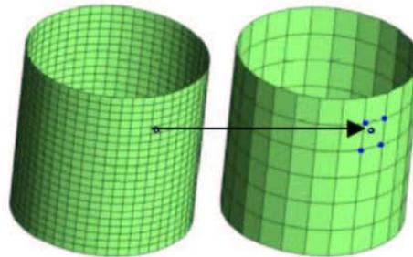
FIG. 1 – Examples of fluid and structure meshes of the interface for data projection and interpolation
