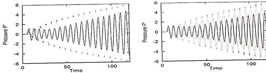
Fig. 9 Time history of pressure  $p'$  evaluated numerically (left) and analytically (right) at centerline (- - -) and at wall (—) for  $\Omega = 2\pi$  and at  $x = \lambda$  with two modes at the inlet.
