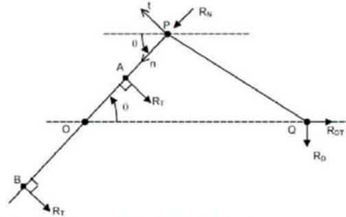
Fig. 6: Free-body diagram of an oscillating piston.
