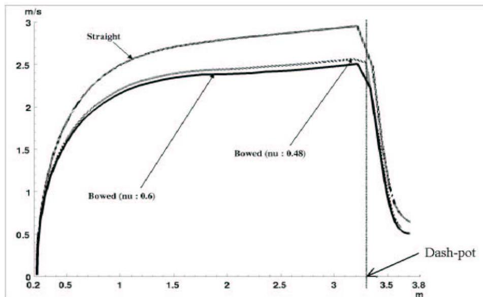
Figure 4 : velocity of the rod according to the altitude. The effect of uncertainty on the friction coefficient is relatively weak compared to the effect of the deflection of the guide.
