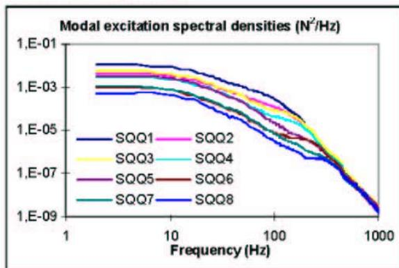
Figure 7: Typical modal excitation spectral densities  $S_{QQ}$
