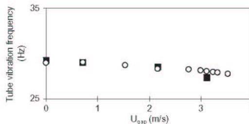
Fig. 12. Tube vibration frequency in flow  $f$  (Hz) in terms of gap velocity  $U_{gap}$  (m/s) estimated numerically (black points) and experimentally by Granger et al. (1993) (white points).
