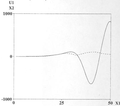
Figure 9: Spatial development of instabilities on axis  $x_2 = 0$  computed with LEE (lines) and with SLEE (points). Velocity  $u'_1$ .
