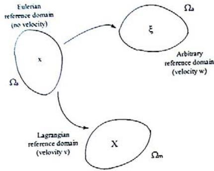
Figure 1 : representation of spatial, material and arbitrary domains  $\Omega_e$ ,  $\Omega_m$  and  $\Omega_a$  whose velocities are respectively 0,  $v$  and  $w$ .
