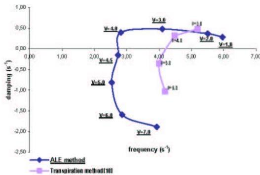
Fig. 7 – Frequency-damping plane for different inlet velocities
