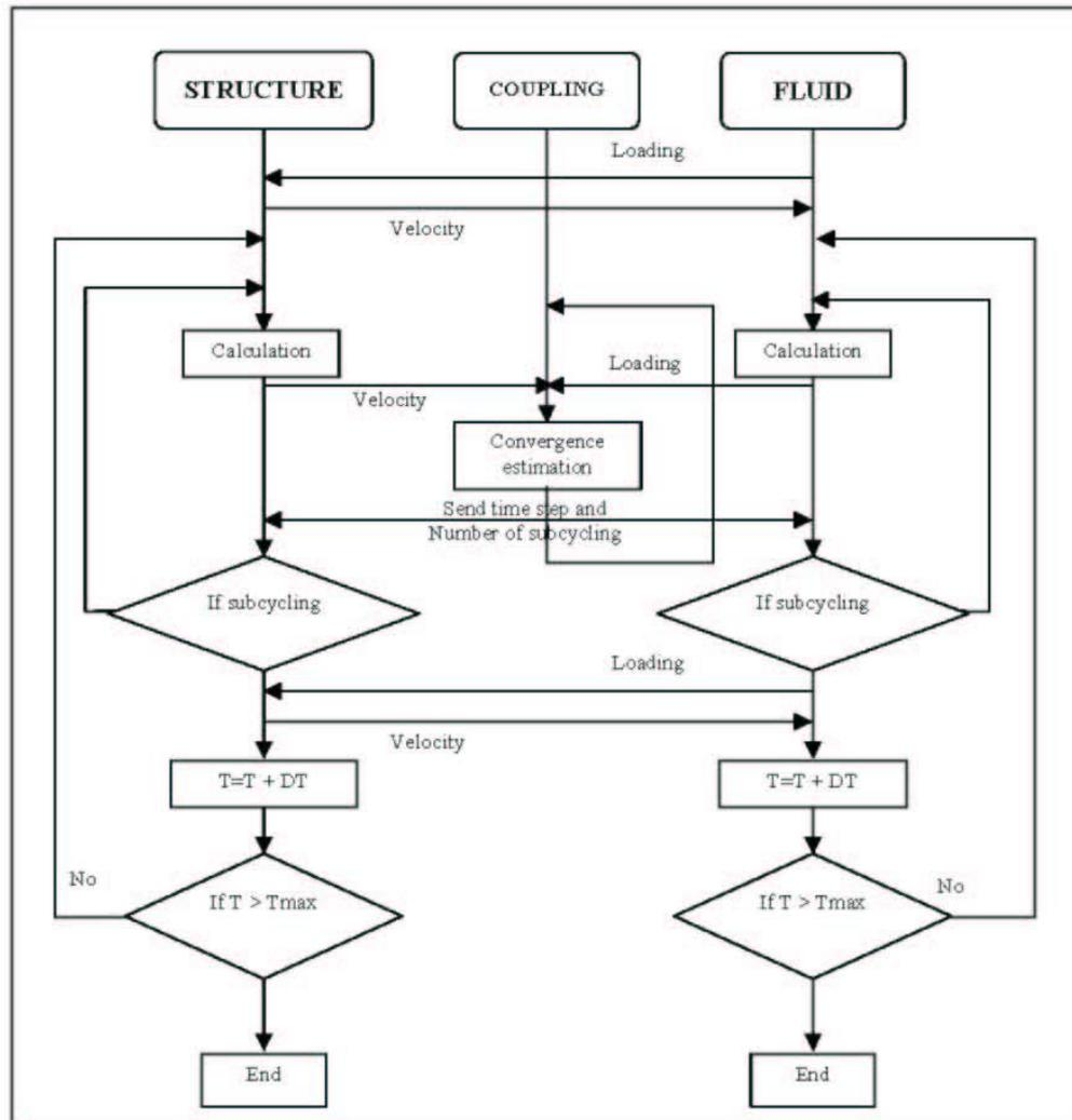
FIG. 2 – Fluid structure code coupling algorithm
