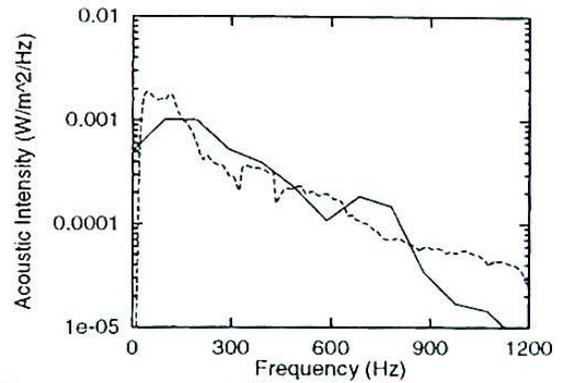
Figure 15: Acoustic intensity spectrum for  $U_0 = 14\text{m/s}$  computed numerically (solid line) and experimentally (dashed line).
