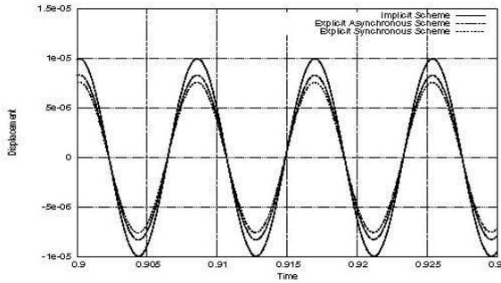
Figure 9. Comparison of structure displacement for three code coupling scheme explicit synchronous, explicit asynchronous and implicit
