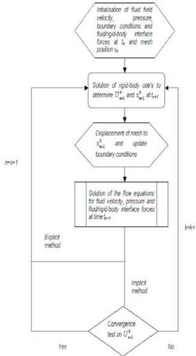
Fig. 3: Flow diagram showing stages of the fluid-structure interaction calculation.
