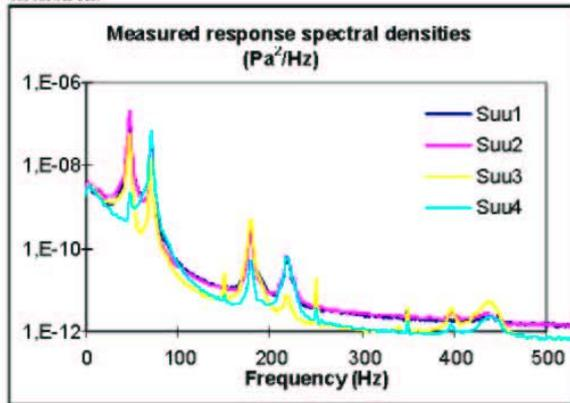
Figure 5: Typical measured response spectral densities  $S_{uu}$  for strain gauges located at one point on the intermittent guidance, for the rod in position E (900 Mwe).
