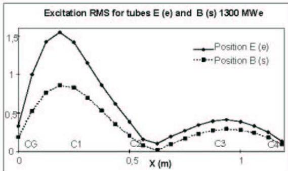
Figure 13 : Comparison of excitation RMS obtained for internal (position E) and external (position B) tubes. 1300 Mwe
