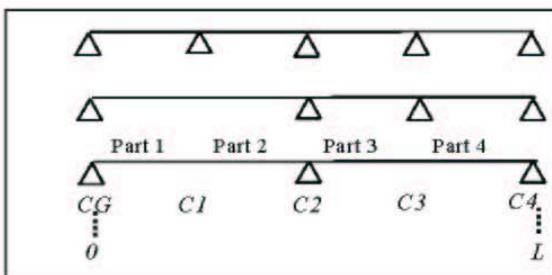
Figure 11: 3 tube support conditions: with 5 supports (top), with 4 supports (middle), with 3 supports (bottom). Supports are located at the continuous guidance top (CG) and at the fourth inferior guide plates of intermittent guidance (C1, C2, C3, C4).
