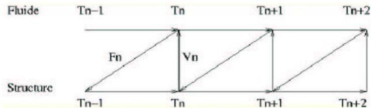
FIG. 3 – Synchronous coupling scheme algorithm
