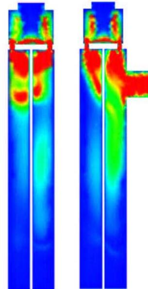
Figure 7 : Mean kinetic turbulent energy deduced from a time-averaged LES for  $t=15s$  in the outlet symmetry plane (right) and in the orthogonal plane (left). Turbulent energy maximal values located near the transverse outlet. Minimal value :  $0 \text{ kgm}^2/\text{s}^2$  (blue colour), artificial maximal value represented on the graphic:  $2,1 \text{ kgm}^2/\text{s}^2$  (red colour).
