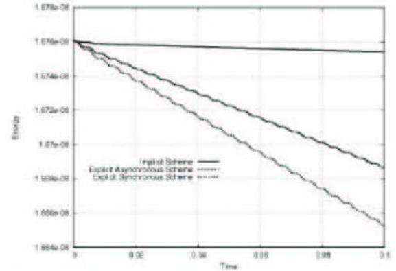
Figure 3 : Comparison of fluid-structure mechanical energy for the three code coupling schemes explicit synchronous, explicit asynchronous and implicit.
