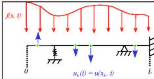
Figure 1: Flexural vibration of a multi-supported beam subjected to a distributed external loading.
