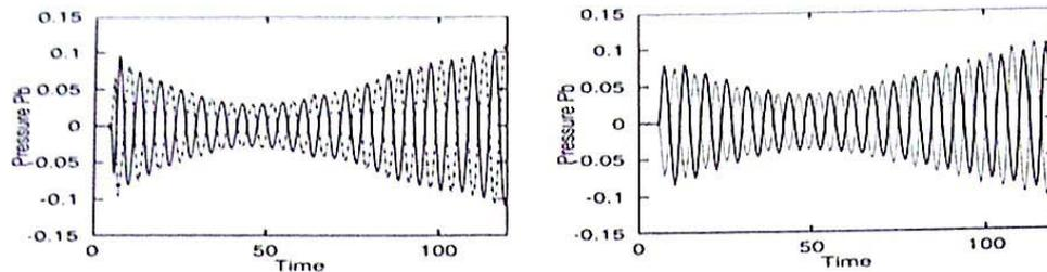
Fig. 11 Time history of pressure  $p_b$  evaluated numerically (left) and analytically (right) with  $M = 0.08$  for  $\Omega = 2\pi$  at  $x = \lambda$  at centerline (---) and at wall (—) with the plane mode at the inlet.
