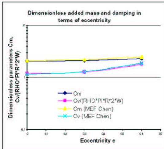
Figure 9 : Dimensionless added mass and damping in terms of eccentricity for eccentric tubes. Comparison of numerical solutions with the numerical partitioned procedure and the numerical monolithic solution in Chen et al. (1987).
