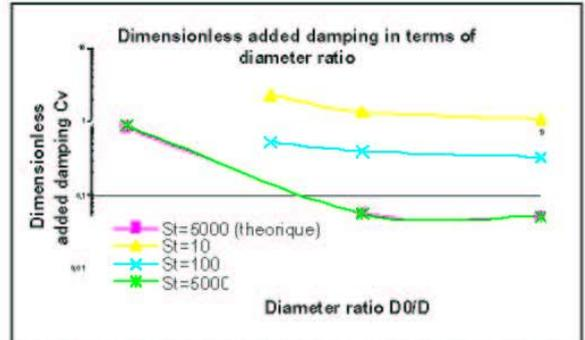
Figure 6 : Dimensionless added damping in terms of diameter ratio for concentric tubes for different Stokes numbers for viscous fluid ( $St = 10, 100, 5000$ ). Comparison of numerical and analytical available solutions.
