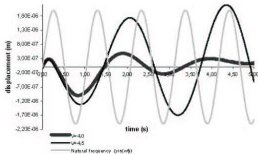
Fig. 8 - Displacement of the end of the structure
