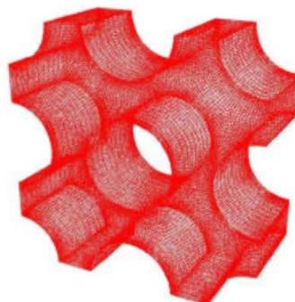
Fig. 10. 3-D mesh of the fluid computational domain at time step  $n = 1$  with a 9-tubes configurations.
