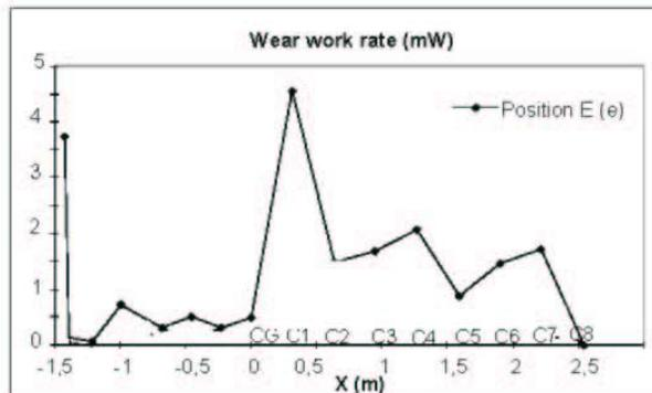
Figure 10 : Wear work rate estimation for the rod in position E (900 Mwe).
