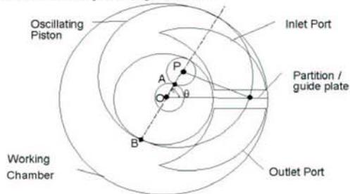
Fig. 5: Schematic of an oscillating piston meter.
