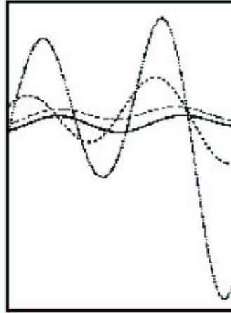
FIG. 11 – Tube displacement of a single flexible tube in a fixed tube bundle in cross flow for several flow velocities obtained with a numerical partitioned procedure (Longatte et al. [6][7]). Stable and unstable tube behaviour above and below the critical flow velocity
