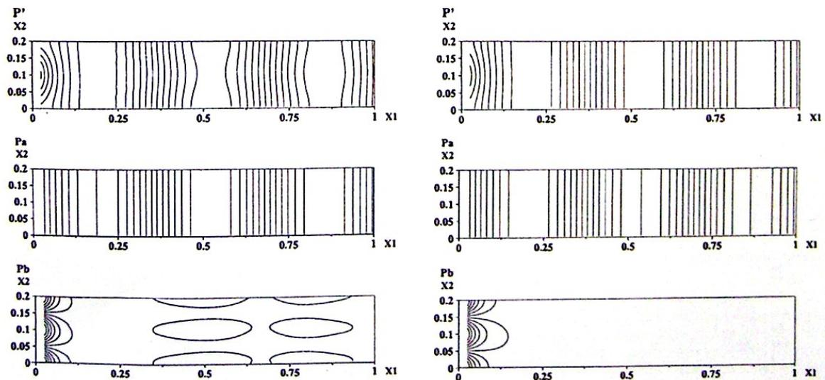
Fig. 3 Components of acoustic first modes evaluated numerically (left) and analytically (right): full solution (top), plane mode  $p_a$  (middle), and nonplane mode  $p_b$  (bottom) for  $\Omega = 2$ , with two modes at the inlet.
