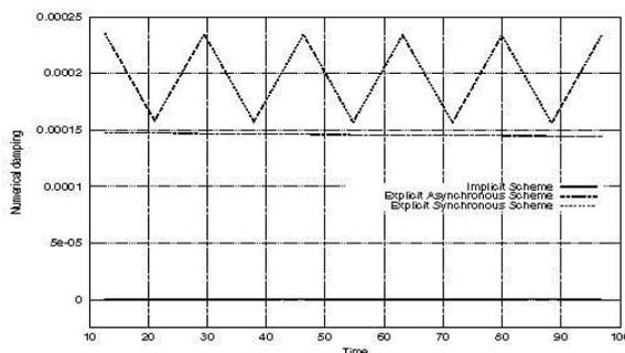
Figure 5. Comparison of numerical damping time evolution for three schemes A, B and C estimated by using tube displacement.
