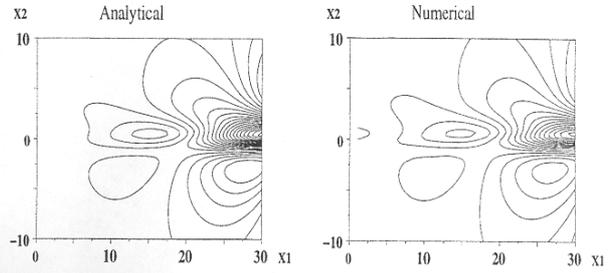
Figure 6: Linear development of unstable modes. Velocity fields estimated numerically with linearized Euler equations (links) and analytically (rights).
