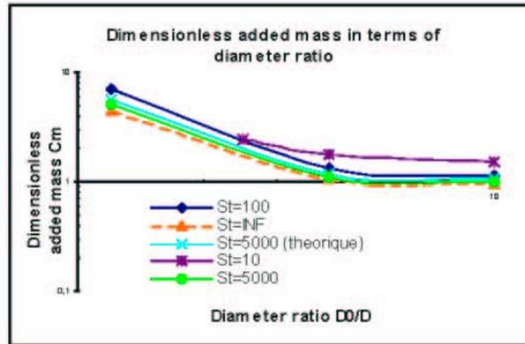
FIG. 6 – Dimensionless added mass depending on internal and external tube diameter ratio for concentric tubes for several Stokes numbers for viscous fluid ( $St = 10, 100, 5000$ ) and for non viscous fluid ( $St = \text{infinity}$ ). Good agreement between numerical results (Longatte et al. [7]) and analytical solutions of Chen [2]
