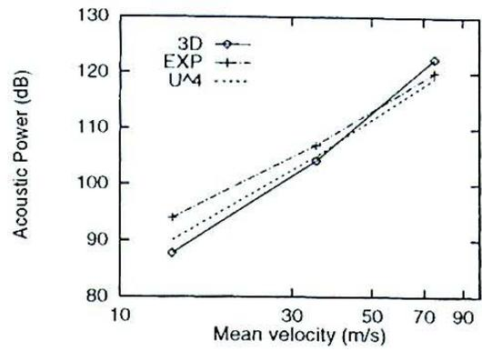
Figure 14: Acoustic power. Comparison of three-dimensional numerical solution, non-dimensional law and experimental data.
