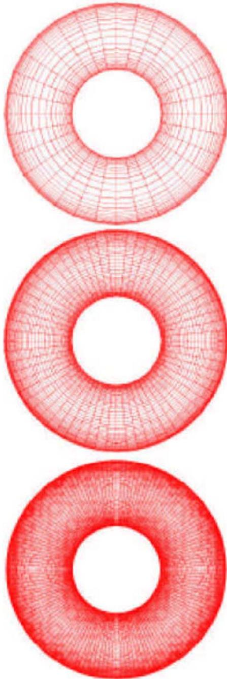
Figure 11. Coarse mesh (896 cells), middle (3712 cells) et fine (16048 cells)
