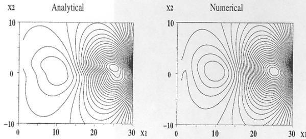
Figure 5: Linear development of unstable mode. Pressure fields estimated numerically with linearized Euler equations (links) and analytically (rights).
