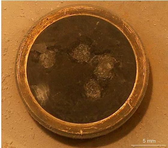
Fig. 5. “Whitening” effect obtained on a soot–ice sample by visible laser irradiation ( $E_{\text{VIS}} = 7 \text{ mJ/pulse}$ ).
