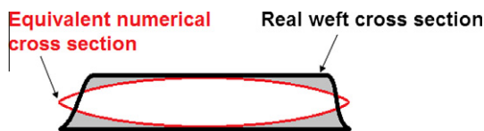
Fig. 12. Equivalent lenticular and real trapezoidal weft cross-sections.
