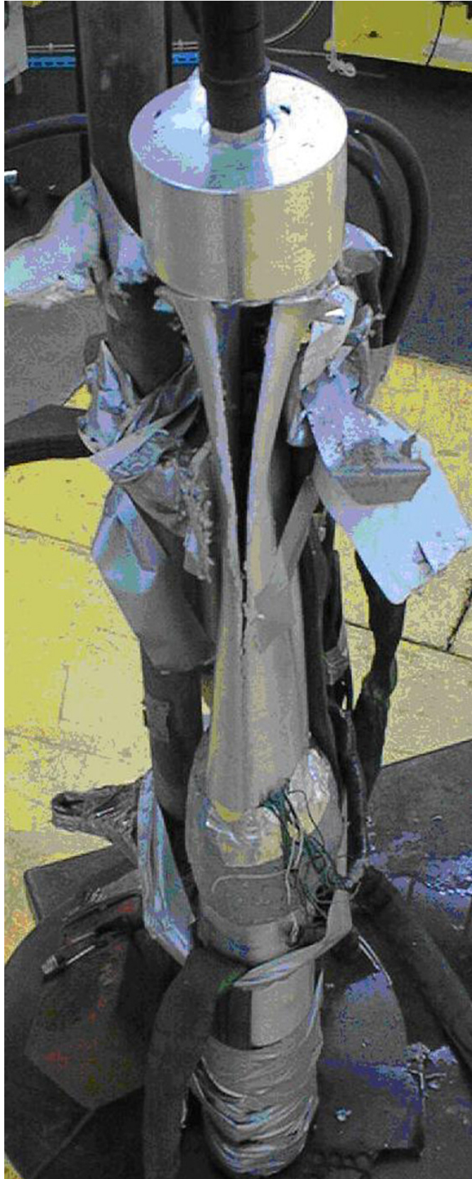
Fig. 6. Collapse of the cylindrical tube.
