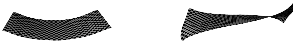
Figure 1.1: Illustration of a key difference between plate theory and shell theory: (Left) A typical deformation of the plate theory is illustrated: the thin object is deformed by transversal loads like its own weight, or a normal pressure on the surface. (Right) Conversely, a shell structure can carry loads in all directions, and therefore can undergo bending, twisting and in-plane deformation.
