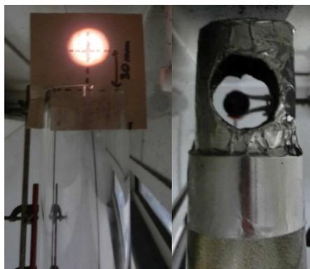
**Figure 47. Light beam / Exhaust end adapter on the top of the mini Steiner tunnel chimney**
