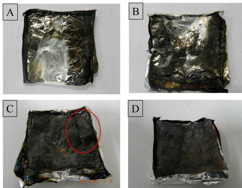
**Figure 56:** Images of the residues of virgin polyamide 6 (A), and PA6 + 5BL (B), 10BL (C) and 20BL (D) coatings after burn testing.
