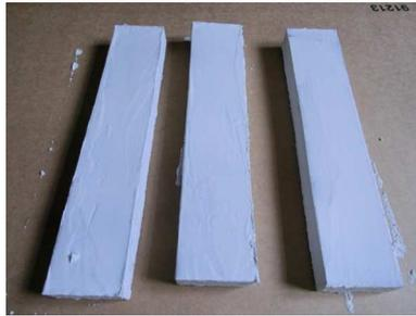
**Figure 44. PET foams coated with the intumescent coating Avicoat**
