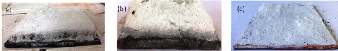
**Figure 78. Pictures of the char after furnace tests (a) reference plate (b) plate after 1 month immersion in distilled water (c) plate after 1 month immersion in salted water**
