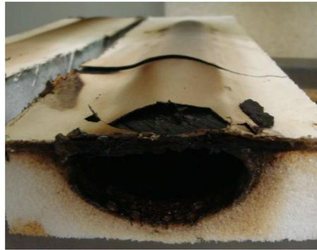
**Figure 49. Residue of PET foam protected by Avicoat in the mini Steiner tunnel**
