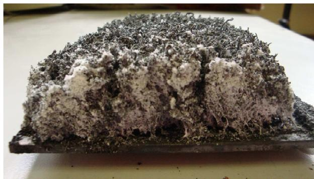
**Figure 5. Intumescent coating protecting a steel plate**
