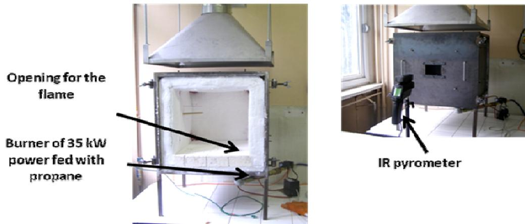
**Figure 28. Small furnace test developed to mimic the UL1709 large scale furnace test**
