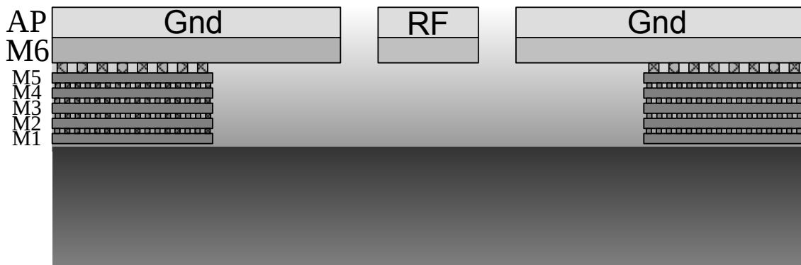
Figure IV-20 Coplanar transmission line in a 65nm CMOS digital BEOL (6 Metal layers)
