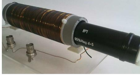
Figure 2.22: Magnetite sample and excitation coil
