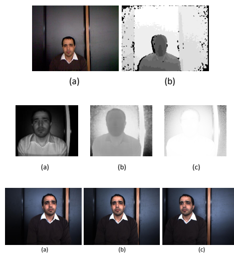
Figure 3.21 – Sample images from the 3 sensors. Top row: infrared sensor images from Kinect: (a) color (b) depth. Middle row: time-of-flight sensor images from SR4000: (a) infrared (b) depth (c) confidence matrix (bright pixels mean high confidence). Bottom row: image triple from the stereo camera Bumblebee XB3.
