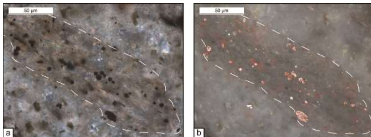
Figure 17 : BOS particle in cement paste ; a) transmitted light, crossed polars b) reflected light
